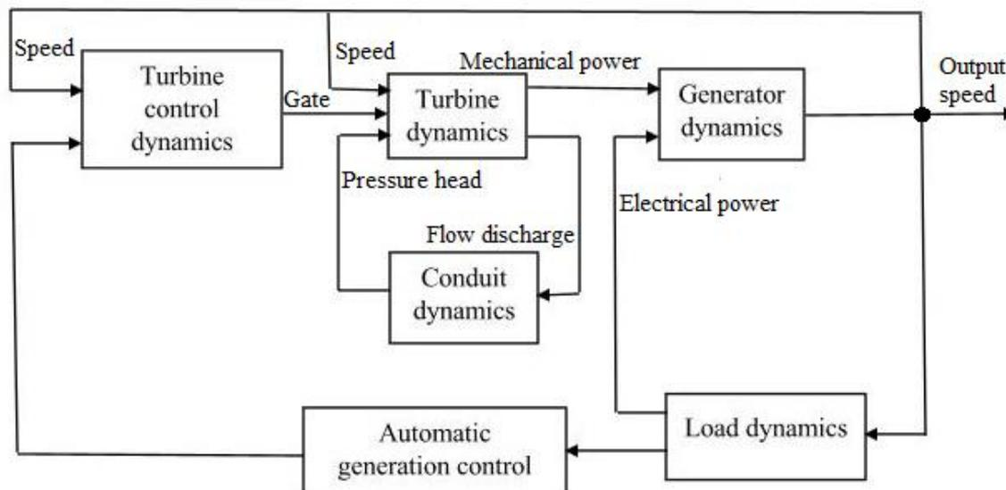
Figure 1.2: Hydropower plants functional block modelling diagrams
