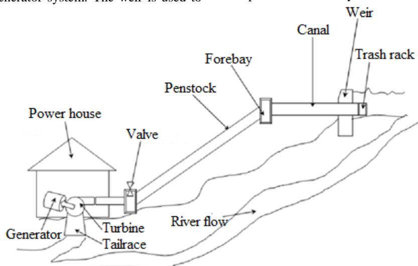
Figure 1.1: Schematic diagram of a micro-hydropower plant [1]
