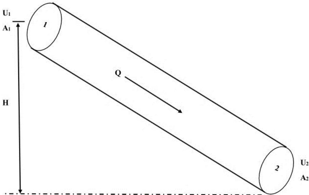
**Figure 2.1:** Water flow discharge through a penstock pipe
