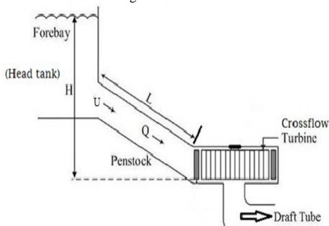
Figure 1.3: Components layout of a hydro turbine system [2]
