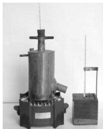
Figure 1: Experimental Setup for the specific heat
