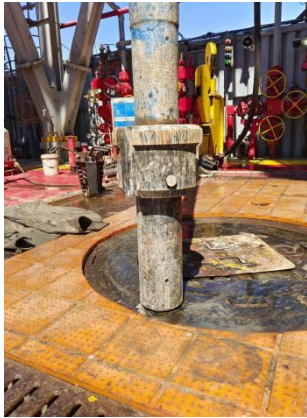
Figure 5: Integrated tool for wellhead flushing and fishing, drilling flushing and fishing sleeve diagram
