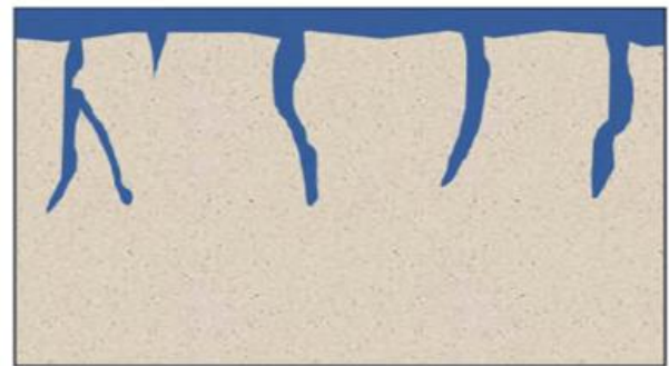
Figure 5: Pore-sealing protection mechanism (Adapted from Ref. [5])
