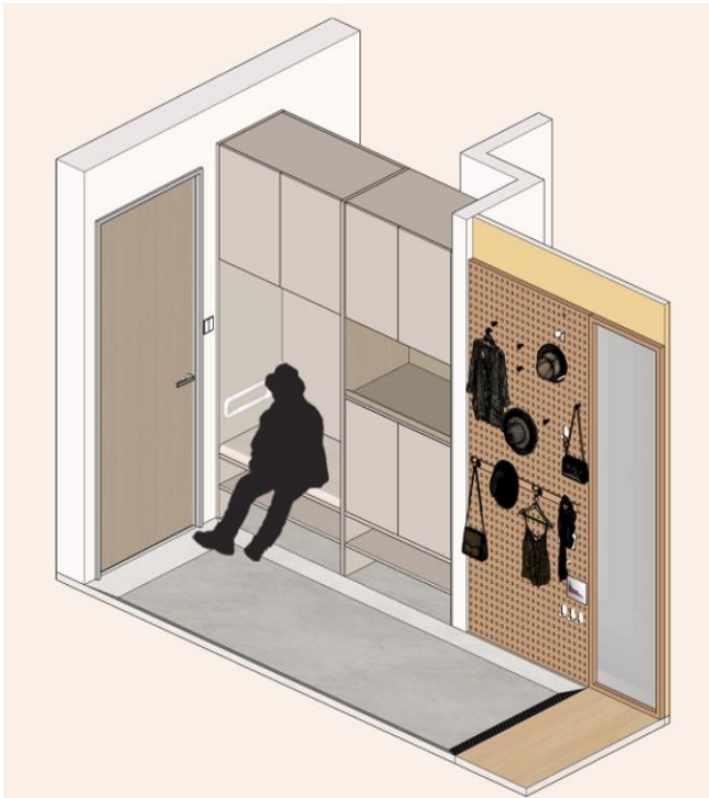
Figure 7: Entrance cabinet and invisible armrest design
