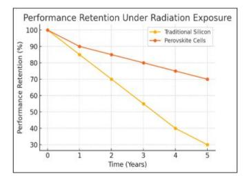
Figure 2 contrasts the radiation resistance of different solar cell improvements under simulated space circumstances. The findings demonstrate that, in comparison to normal crystalline solar cells, perovskite solar cells exhibit a gradual deterioration in quality. Alternatively, when the cell is subjected to ionising radiation. Perovskite cells maintained over 85% of their initial performance following five erroneous exposures, in contrast to crystalline cells. Only
