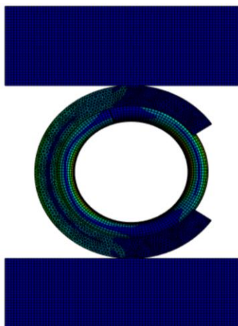
Figure 3: Finite element analysis of C - shaped metal seal ring
