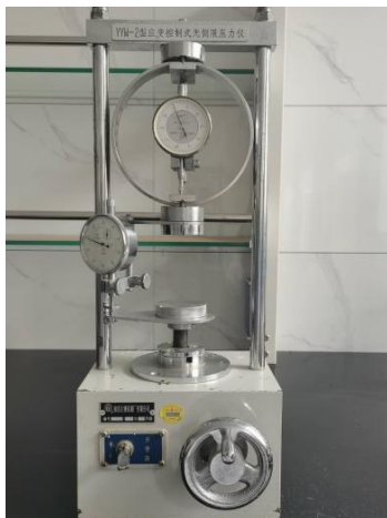
Figure 2: YYW- 2 strain-controlled unconfined manometer.
