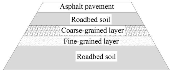
**Figure 7:** Covers with capillary barrier effects for subgrade
