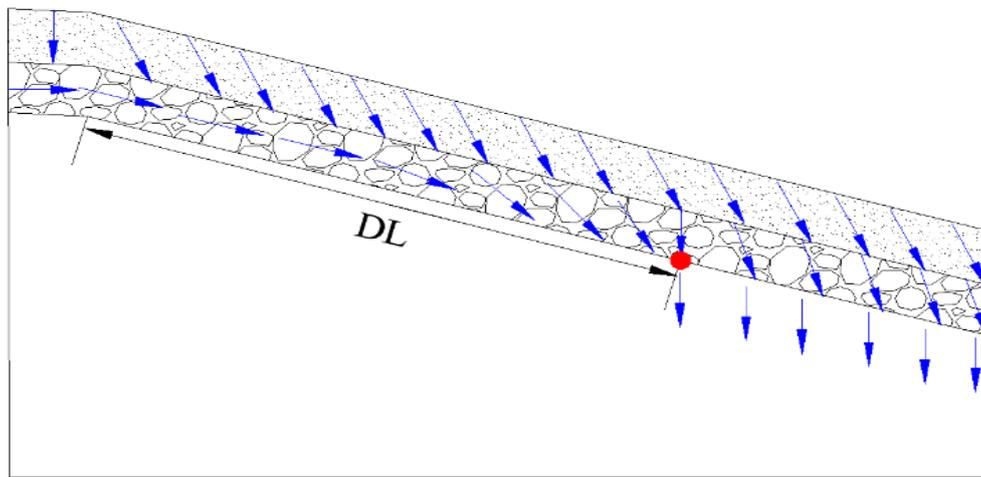
**Figure 2:** Schematic representation of water movement in an inclined capillary barrier
