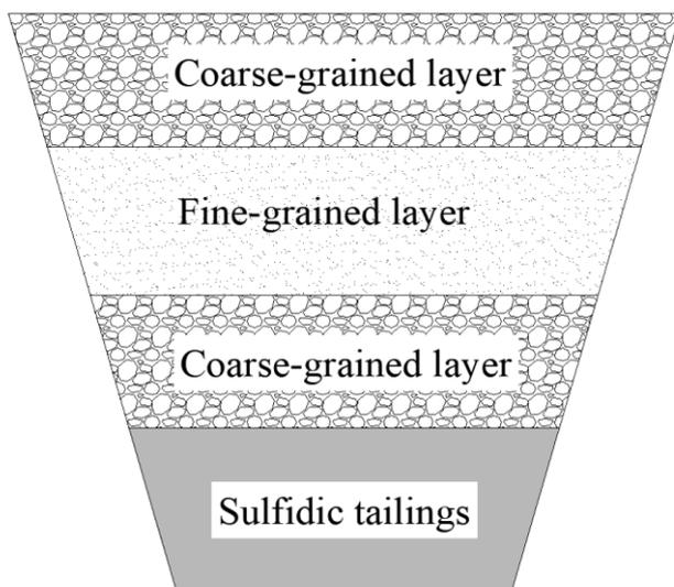
**Figure 5:** Covers with capillary barrier effects of acid tailings ponds
