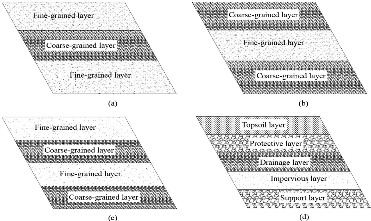
**Figure 3:** Covers with capillary barrier effects structure (a) three layers of fine-coarse-fine; (b) three layers of coarse-fine-coarse; (c) four layers; (d) five layers
