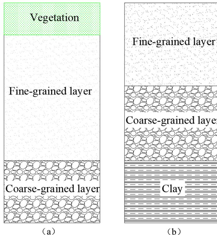
**Figure 4:** (a) Capillary barrier evapotranspiration covers; (b) New three-layer landfill cover system
