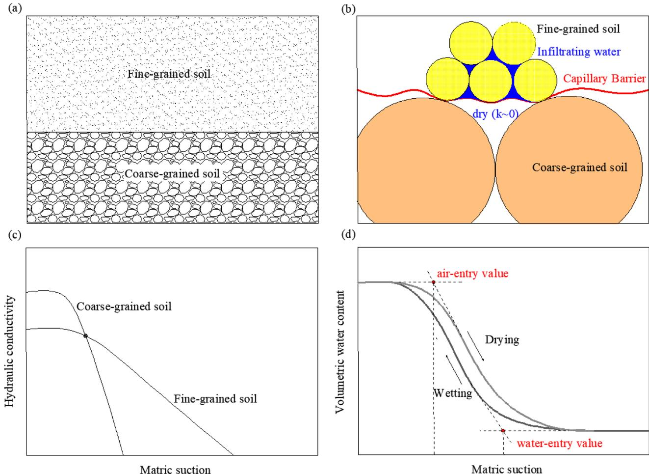
**Figure 1:** (a) Basic structure of the capillary barrier; (b) Capillary barrier at the interface between soils with different conductivity; (c) Hydraulic conductivity of coarse- and fine-grained soils in capillary barrier structures; (d) Soil-water characteristic curve for coarse grains
