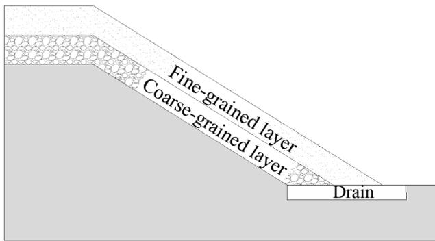
**Figure 6:** Slope covers with capillary barrier effects
