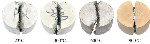
Figure 6: The failure modes of splitting tensile resistance of UHPC before and after high temperature treatment
