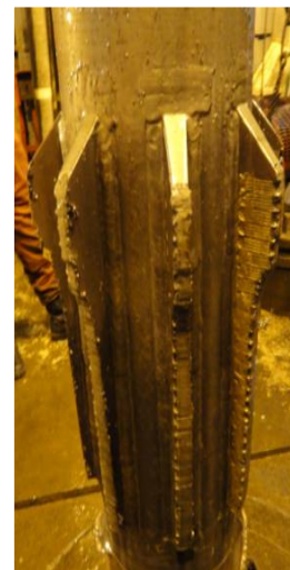
Figure 7: Shoe Grinding for Collar Hole Out of Well
