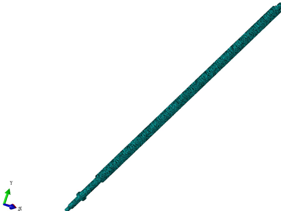
Figure 7: Finite Element Mesh Model of the screw
