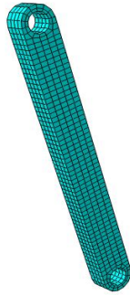
Figure 5: Finite Element Mesh Model of the connecting rod
