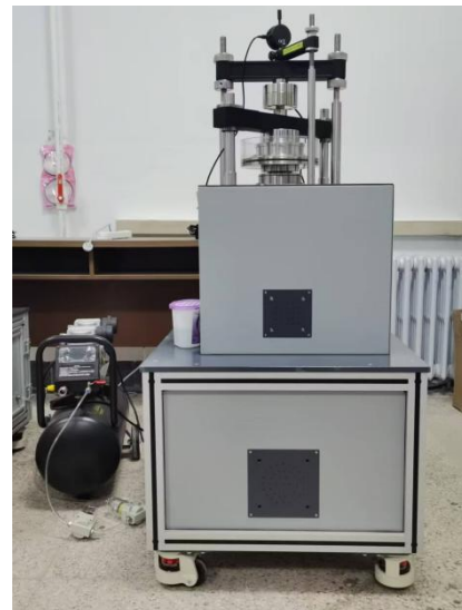
Figure 2: TT-RSA-10F Automatic Servo-Controlled Ring Shear apparatus
