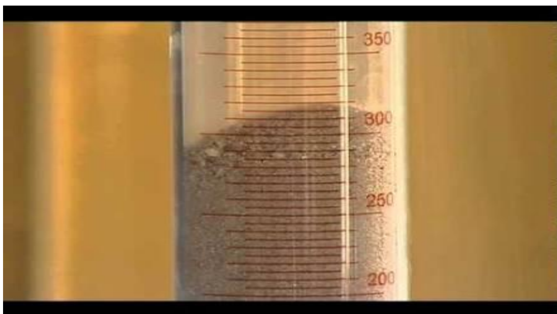
Figure 9: Bulking of sand
