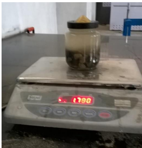
Figure 10: Specific gravity of coarse aggregate
