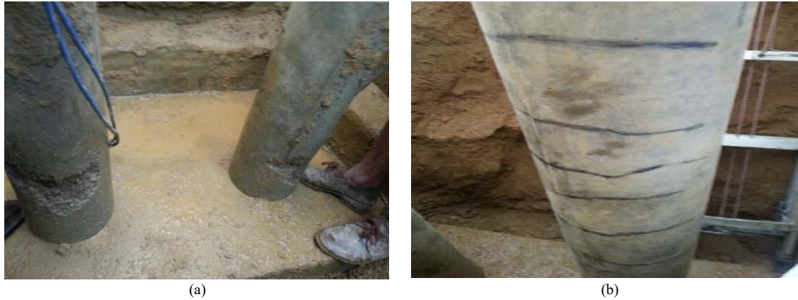
Figure 5: The test processes: (a) before loading; (b) fractures on pile body
