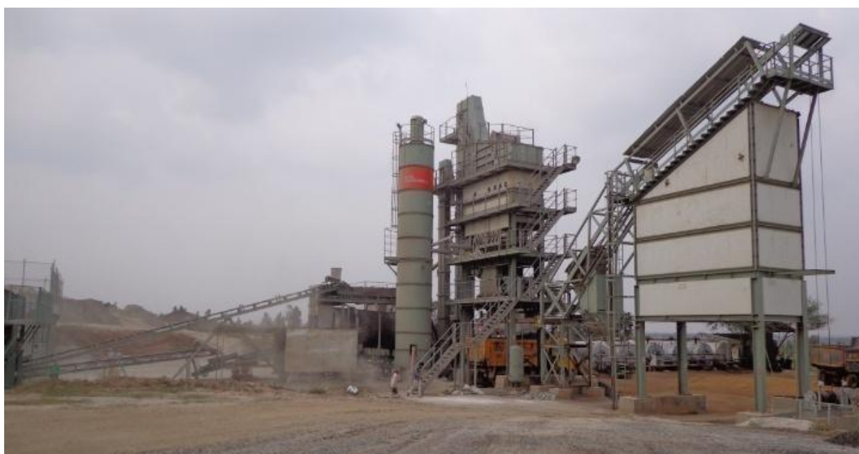
Figure 2.4: Asphalt batch plant with RAP in feed for hot recycling
