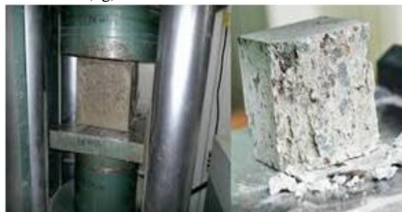
Compressive test of sample
