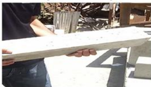
Beam Specimen for Flexure Test
