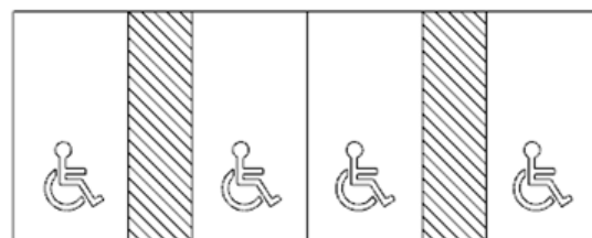
Figure 14: Disabilities Signage at the car park
