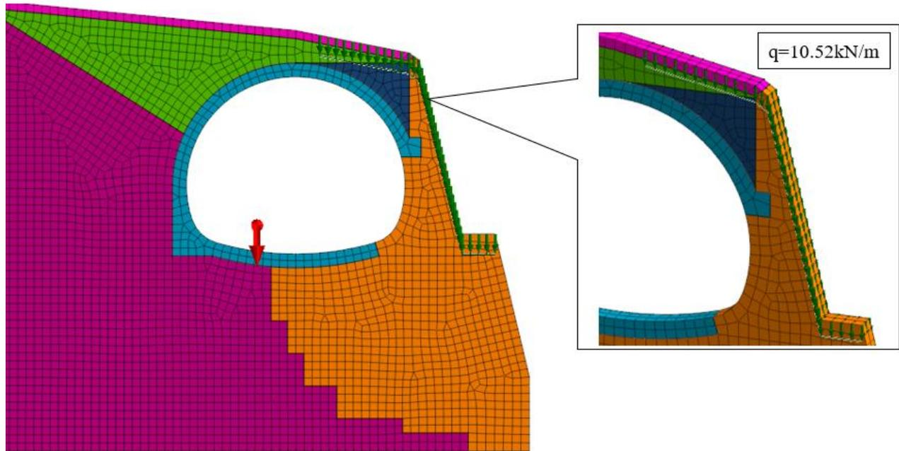
Figure 5: Schematic Diagram of Impact Load Application
