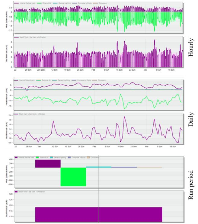
**Figure 3: Air Change Per Hour (ACH) Calculations of the Base Case**
