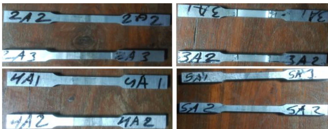
Figure 7: Specimens are cut as per requirement by wire EDM
