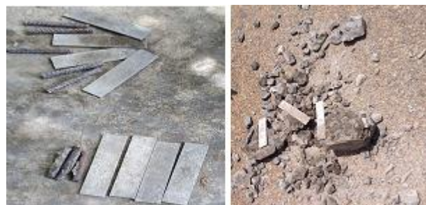
Figure 4: Metal samples taken out of the concrete
