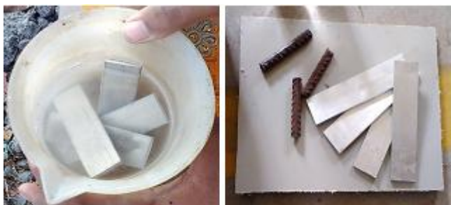
Figure 1: Metal Samples coated with corrosion inhibitor
