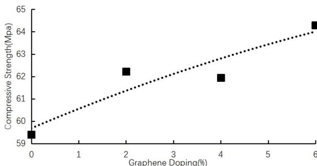
**Figure 3:** Compressive strength curve of graphene doping
