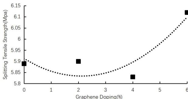
**Figure 5:** Graphene doping splitting tensile strength curve
