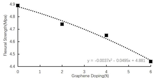
**Figure 4:** Graphene doping flexural strength curve
