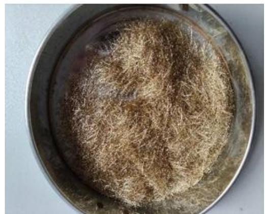
Figure 2: Sheared steel fiber
