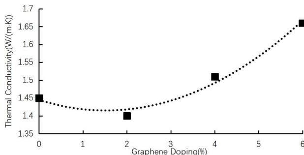
**Figure 6:** Graphene doping thermal conductivity curve
