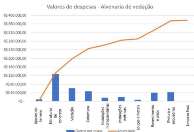
Figure 2: Expense values - Sealing masonry.
